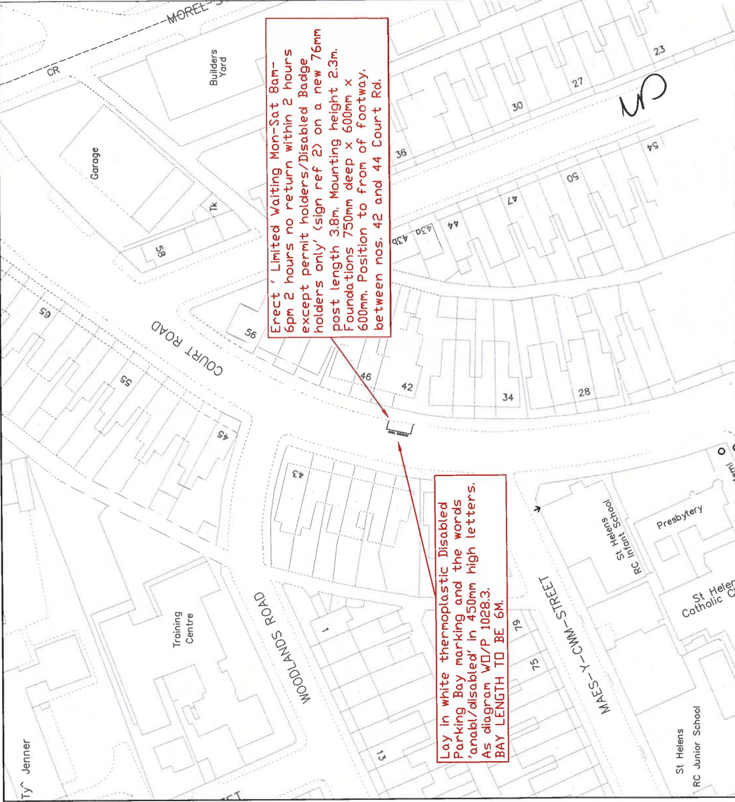
Erect ' Limited Waiting Mon-Sat 8am-6pm 2 hours no return within 2 hours except permit holders./Disabled Badge holders only' (sign ref 2) on a new 76mm post length 3.8m. Mounting height 2.3m. Foundations 750mm deep x 600mm x 600mm. Position to from of footway, between nos. 42 and 44 Court Rd.
